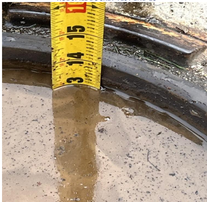
RUL SPILL BUCKET TEST END 13"
