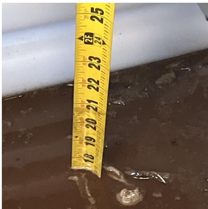
DISP 7/8 SUMP TEST START 17.5"
