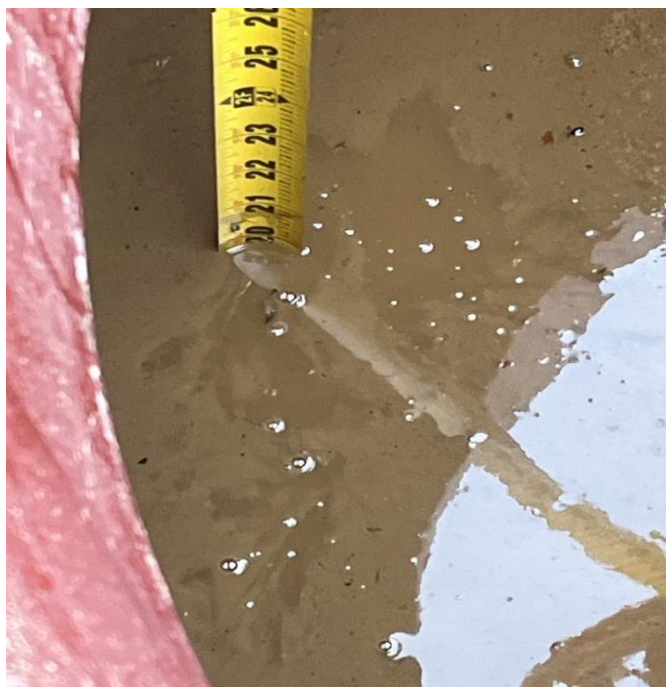
KER STP SUMP TEST START 20"
