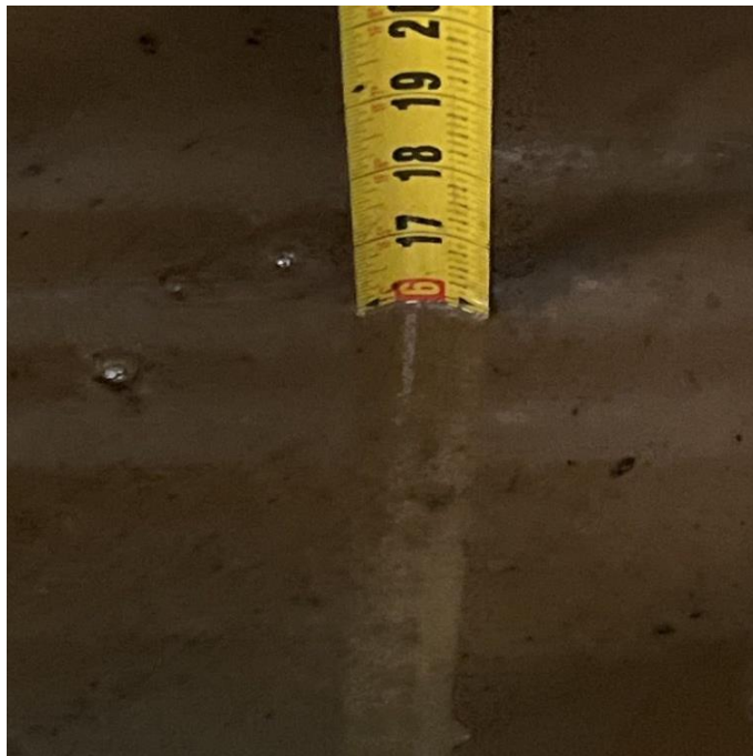
DISP 1/2 SUMP TEST START 16"
