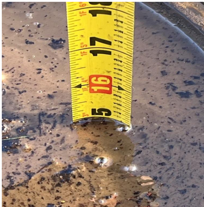
DSL SPILL BUCKET TEST START 15"
