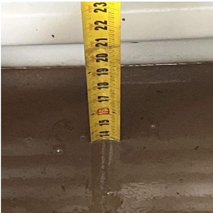
DISP 5/6 SUMP TEST START 13.75"
