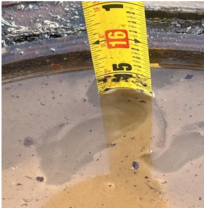
KER SPILL BUCKET TEST START 14.5"
