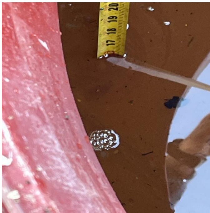
PUL STP SUMP TEST START 16"
