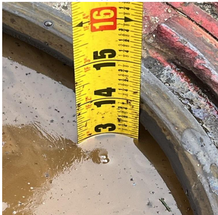
PUL SPILL BUCKET TEST END 13"
