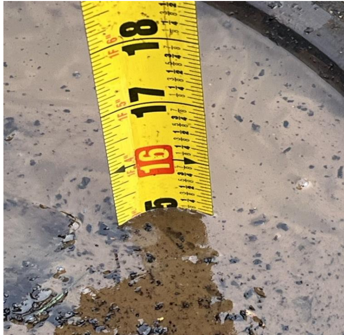
DSL SPILL BUCKET TEST END 15"
