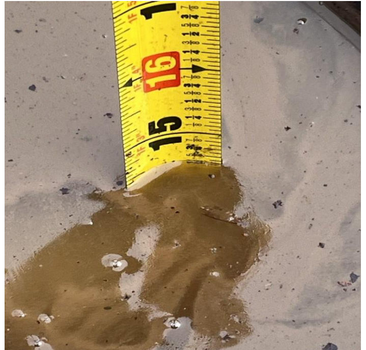
KER SPILL BUCKET TEST END 14.5"
