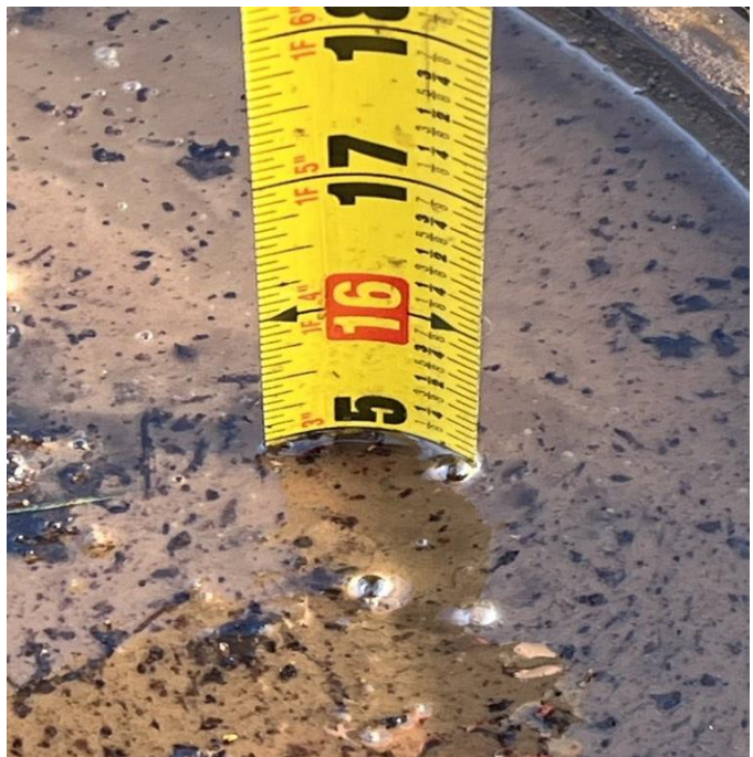
DSL SPILL BUCKET TEST START 15"
