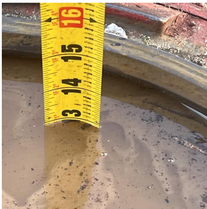
PUL SPILL BUCKET TEST START 13"
