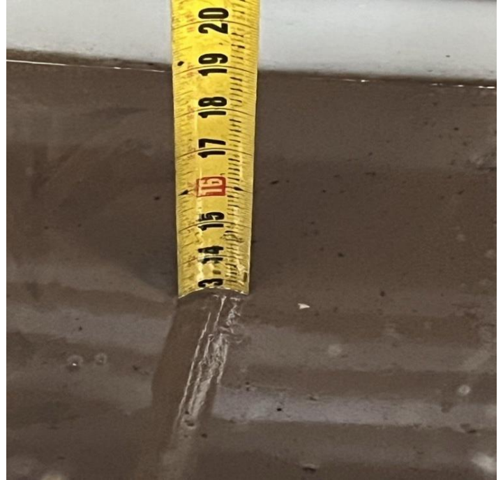
DISP 3/4 SUMP TEST END 13"
