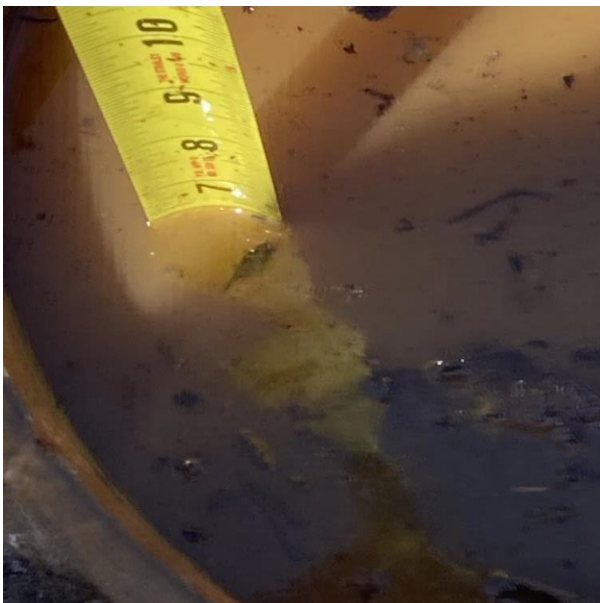
RUL1 SPILL BUCKET TEST START 6.5"
