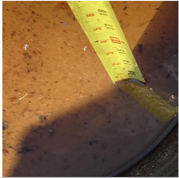
KER SPILL BUCKET TEST END 14"
