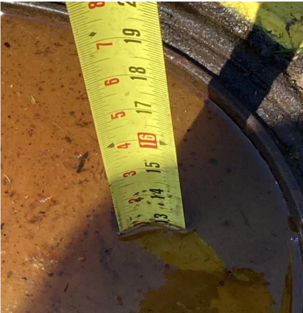
KER SPILL BUCKET TEST START 14"
