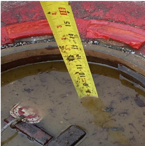
PUL SPILL BUCKET TEST START 7.5"
