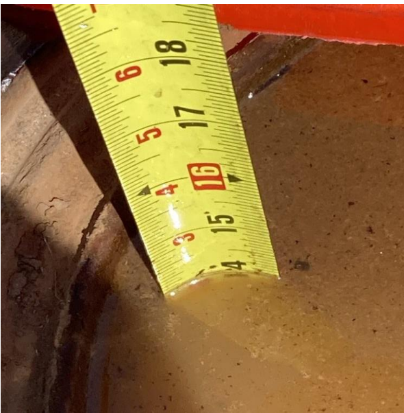
KER SPILL BUCKET TEST START 14"
