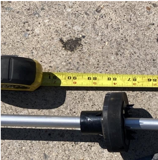
RUL1 SPILL BUCKET TEST START 6.5"
