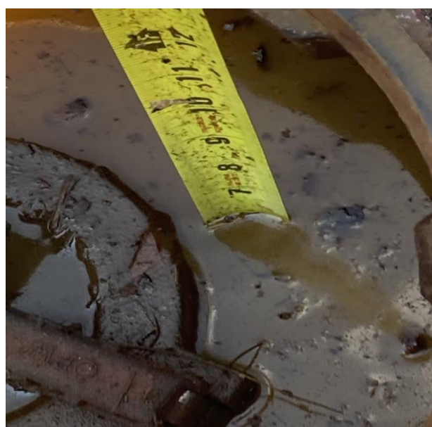
PUL SPILL BUCKET TEST END 6"
