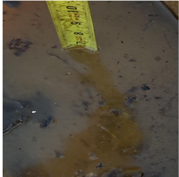
RUL1 SPILL BUCKET TEST END 6.5"
