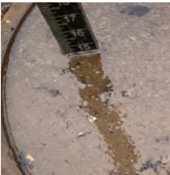
PUL SPILL BUCKET TEST START 14.5"
